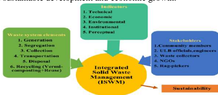
Figure 1: Dimensions of integrated solid waste management Source: Adapted from Scheinberg (2011)
